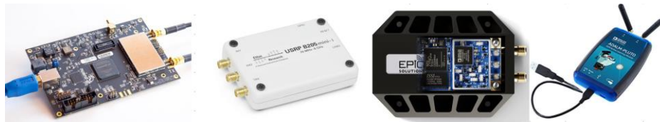
Fig. 5. SDR Devices from left to right a) BladeRF, b) USRP B205, c) Matchstiq Z2, d) Adalm Pluto Transmitter.
