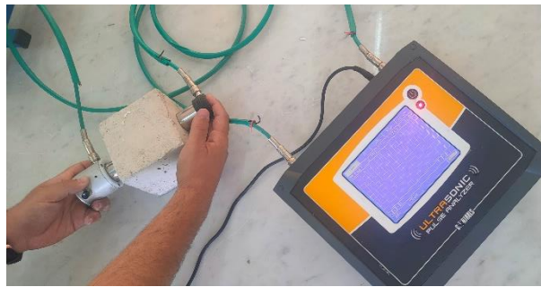
Fig. 3. Measurements by ultrasonic device.
