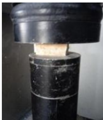
Figure 6: Testing for compression by crush
