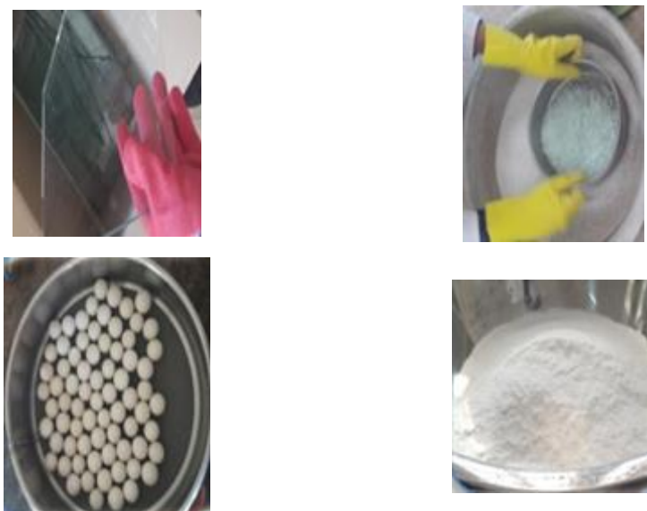
Figure 3: the steps to obtain the glass powder
